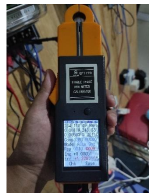
Gambar 2 Alat Ukur Single Phase kWh Meter Calibrator
